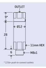
Note: ZEM 32 Series injectors can be used with manifolds (see page 24) or tee fittings (part # 22564).
